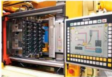
H-PET AE offers a complete system solution for lower volume preform manufacturing.
